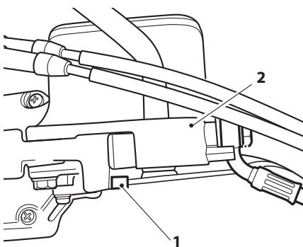
1. Brake light switch connections (Rocket III Touring shown)
