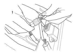
1. Rear light unit wiring connector
