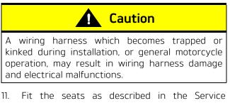
II. Fit the seats as described in the Service Manual. Make sure that the harness for the heated seat does not become trapped between the seat and the frame.
