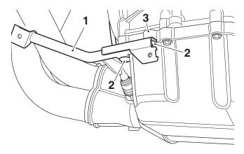
7. Fit the bung from the kit to the catalytic converter heat shield fixing position in the orientation shown.
