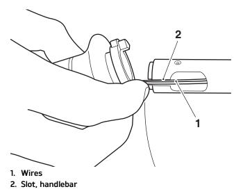
62. Make sure there is enough slack in the wires for the twist grip to rotate and the wires not to become trapped.
