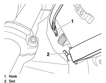
6. Fit the rear hooks to the cut out provided in the fuel tank flange.
