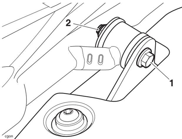
1. Silencer mounting bracket fixing
