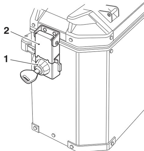
1. Lock barrel - unlock position
