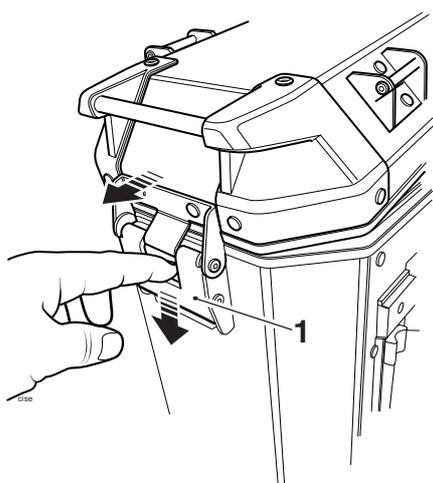
**1. Pannier lid hinge quick-release mechanism**
